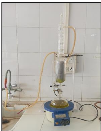
Fig No. 2: Extraction by soxhlet apparatus.
