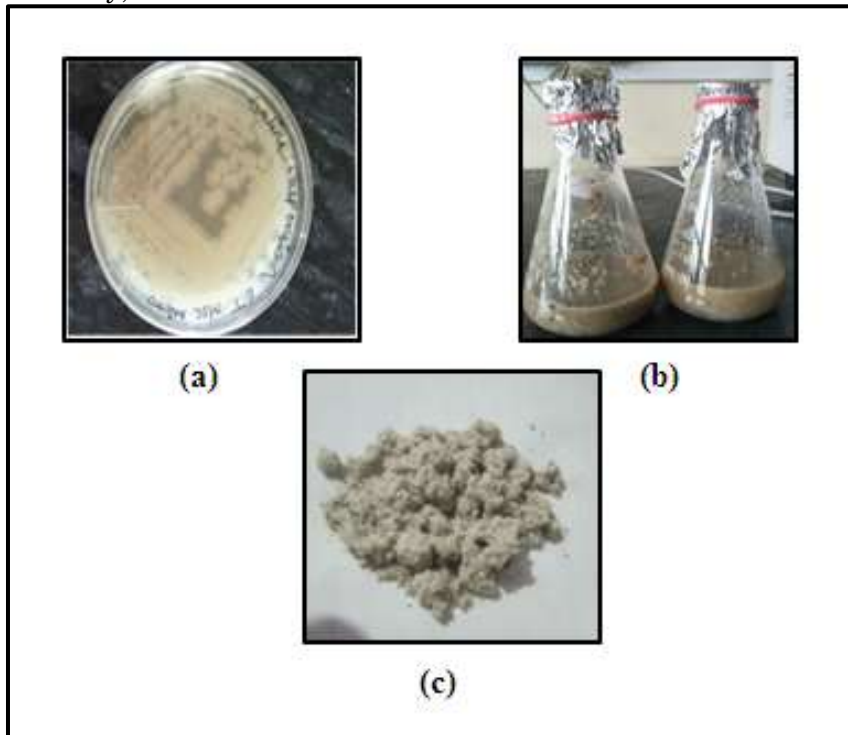
Figure 1: Stages of PHB production (a) Isolated Bacillus thuringiensis (b) Fermented broth of waste residue (c) Extracted PHB granules.
