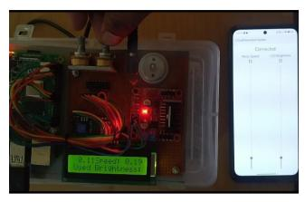
**Dual Control Functionality:** Users have the ability to independently adjust the RPM of the DC motor and the brightness of the OLED display using the two potentiometers. This provides fine-grained control over both parameters, allowing for precise adjustments according to the user's preferences or requirements
