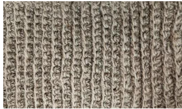
Fig No. 1: Stockinette Knit Structure
