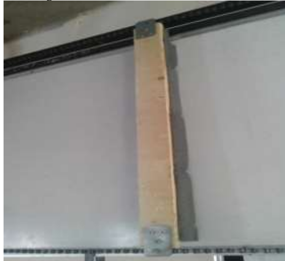
Fig3: Automatic white board cleaner If the command given through mobile application is backward, Shaft moves in the backward direction and motor running in the anti-clockwise direction.
