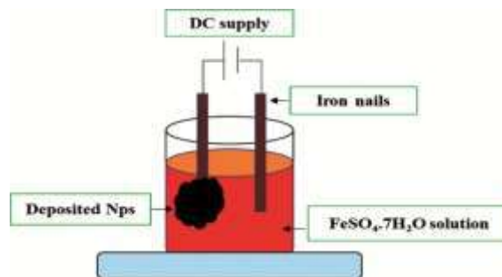
Fig. 1: Electrochemical setup for the preparation of iron oxidenanoparticles.
