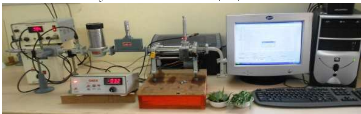
Photograph of automated x-band microwave bench setup for measurement of dielectric constant of tree leaves.
