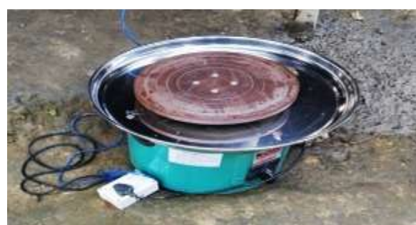
P7: Device of electric wheel to reduce the time and effort of potters.
