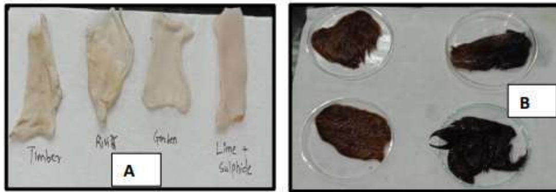
Figure 6: Dehairing of Goat Skin Using Extracted Crude Enzyme from Isolates GS, RS, TS A) Goat Skin Treated with Crude Enzyme B) Untreated Goat Skin
