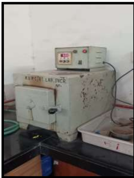
Fig.2 : Ashing of Marigold flower in the furnace at 500°C
