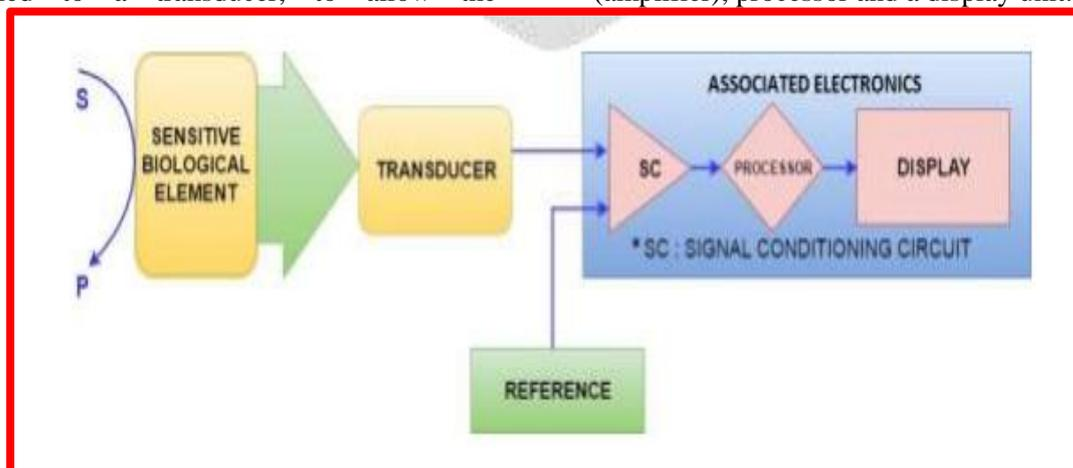
**Fig -1: schematic diagram showing main components of a biosensor**
