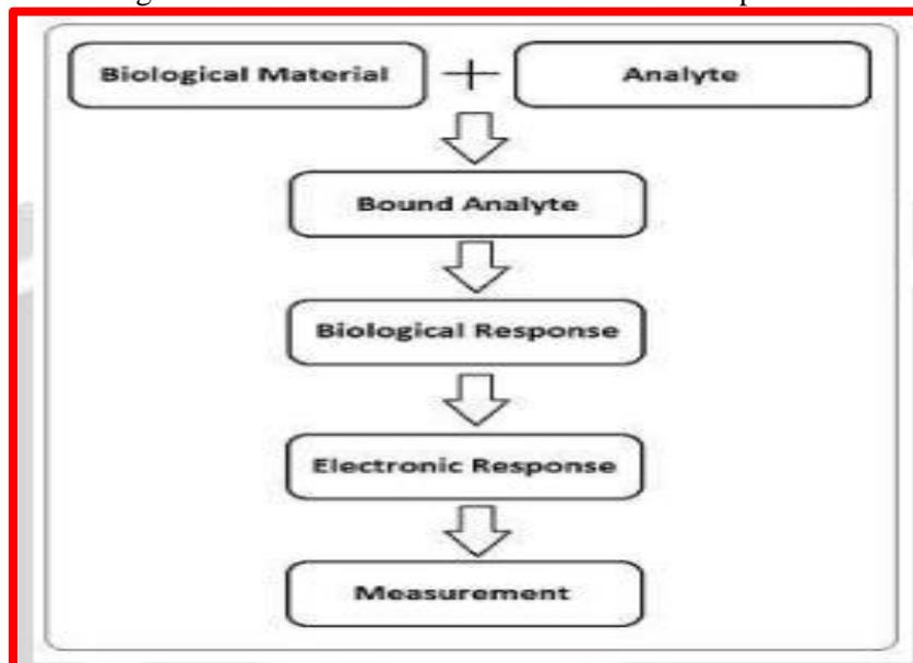
Fig -2: measurement flow for a biosensor
