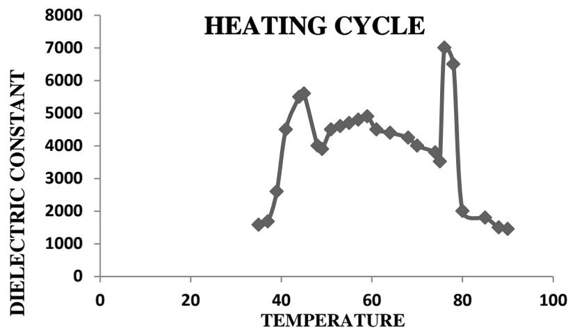
**FIG 1. TEMPERATURE VARIATION OF DIELECTRIC CONSTANT OF  $\text{Cd}(\text{C}_2\text{H}_3\text{O}_2)_2 \cdot 2\text{H}_2\text{O} + \text{Silver Oxide}$**
