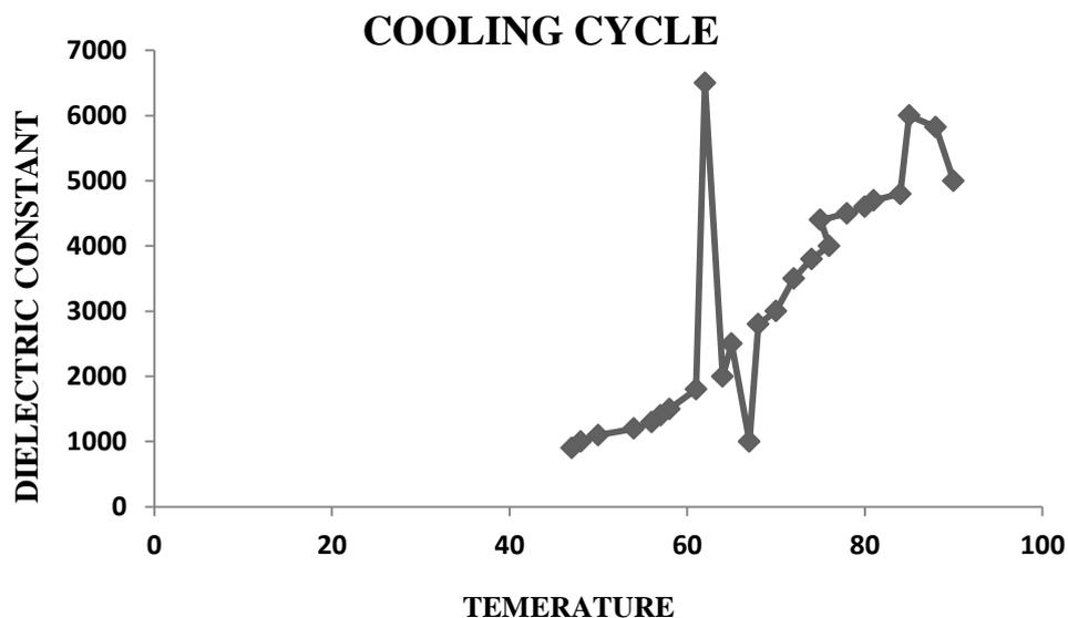
**FIG 2. TEMPERATURE VARIATION OF DIELECTRIC CONSTANT OF  $\text{Cd}(\text{C}_2\text{H}_3\text{O}_2)_2 \cdot 2\text{H}_2\text{O} + \text{Silver Oxide}$**
