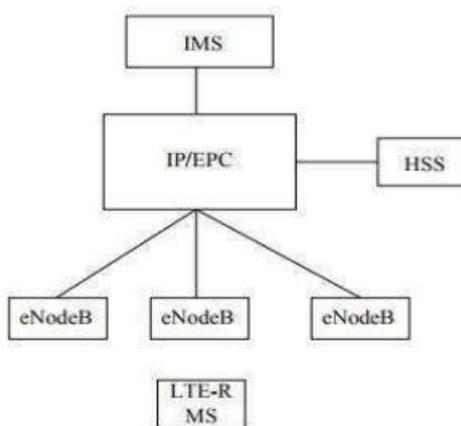
Figure 1. network architecture of LTE-R
