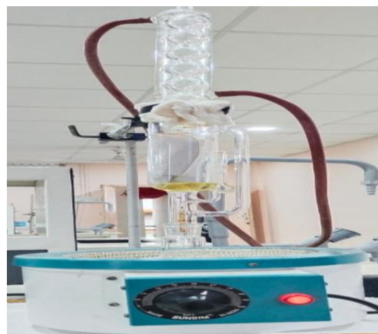
Fig.4. Soxhlet Method (Extraction Process)
