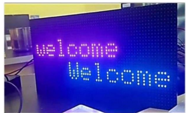
Fig 4 LED matrix display output of the proposed smart e-circular notification system.
