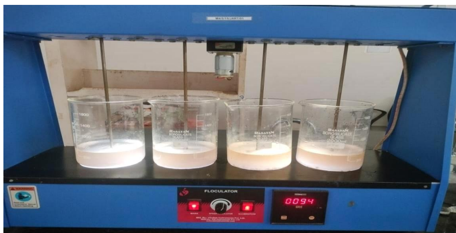
Fig no-4.1. Jar Test with Banana Peel Extract Table no-2. moringa oleifera with extract
